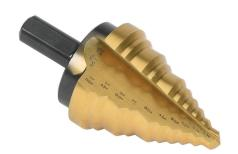
Viking step drill bit, 7/8in to 1-3/8in, size #12, 5 steps, split point, high-speed steel (HSS), Titanium-Nitride (TiN) coated finish, 3/8in diameter 3-flat shank, 2.8in (71mm) overall length.
