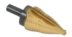
Viking step drill bit, 1/4in to 1-1/8in, size 1/4A, 16 steps, split point, high-speed steel (HSS), Titanium-Nitride (TiN) coated finish, 3/8in diameter 3-flat shank, 3.0in (76mm) overall length.
