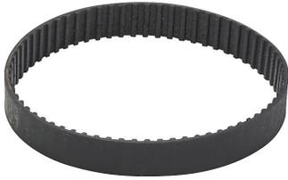
SureMotion timing belt, 0.08in MXL pitch, 1/4in wide, 68 tooth, 5.4in pitch length (circumference), neoprene, fiberglass reinforced. Package of 3.
