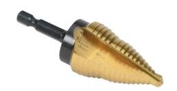
Viking step drill bit, 1/4in to 1-1/8in, size 1/4A, 16 steps, split point, high-speed steel (HSS), Titanium-Nitride (TiN) coated finish, 1/4in hex shank, 3in (76mm) overall length.
