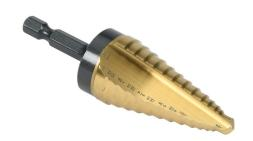
Viking step drill bit, 1/4in to 1in, size #2, 8 steps, split point, high-speed steel (HSS), Titanium-Nitride (TiN) coated finish, 1/4in hex shank, 3in (76mm) overall length.
