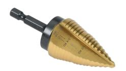
Viking step drill bit, 7/8in to 1-1/8in, size #11, 2 steps, split point, high-speed steel (HSS), Titanium-Nitride (TiN) coated finish, 1/4in hex shank, 2.8in (71mm) overall length.
