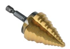
Viking step drill bit, 7/8in to 1-3/8in, size #12, 5 steps, split point, high-speed steel (HSS), Titanium-Nitride (TiN) coated finish, 1/4in hex shank, 2.8in (71mm) overall length.
