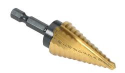
Viking step drill bit, 3/16in to 7/8in, size #8, 12 steps, split point, high-speed steel (HSS), Titanium-Nitride (TiN) coated finish, 1/4in hex shank, 2.8in (71mm) overall length.
