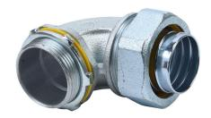
Halex fitting, liquid-tight, malleable iron, 90-degree, 1-1/2in trade size, compression conduit connection, zinc electro-plated finish. Package of 2. For use with LFMC and NM-Type B electrical conduit. Sealing washer and locknut included.
