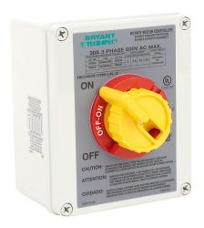
Bryant manual motor controller, enclosed, 30A, 600 VAC, 3-pole, 20hp, wall mount, thermoplastic housing, NEMA 4X, UL 508 rated.
