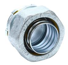
Halex fitting, liquid-tight, malleable iron, straight, 1-1/4in trade size, compression conduit connection, zinc electro-plated finish. Package of 2. For use with LFMC and NM-Type B electrical conduit. Sealing washer and locknut included.
