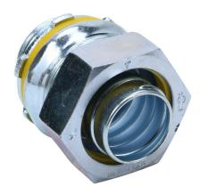
Halex fitting, liquid-tight, malleable iron, straight, 1in trade size, compression conduit connection, zinc electro-plated finish. Package of 5. For use with LFMC and NM-Type B electrical conduit. Sealing washer and locknut included.
