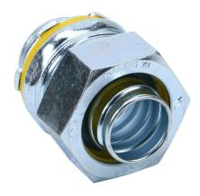
Halex fitting, liquid-tight, malleable iron, straight, 3/4in trade size, compression conduit connection, zinc electro-plated finish.
