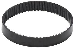
SureMotion timing belt, 0.08in MXL pitch, 1/4in wide, 64 tooth, 5.1in pitch length (circumference), polyurethane, polyester reinforced. Package of 3.
