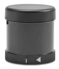
WERMA siren element, 100 dB at 1m, 1.6 kHz to 3.4 kHz tone frequency, (7) selectable tone(s), 24 VDC, polycarbonate housing, black, IP65. For use with WERMA 70mm stack light elements.
