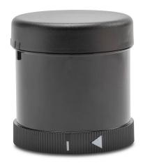
WERMA buzzer element, 85 dB at 1m, 1.8 kHz tone frequency, continuous/pulse tone(s), 24 VAC/VDC, polycarbonate housing, black, IP65. For use with WERMA 70mm stack light elements.
