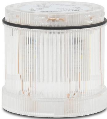
WERMA LED light element, 70mm diameter, clear/white, blinking (1 Hz ON for 550ms) light function, 24 VAC/VDC, clear lens, IP65.
