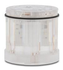
WERMA LED light element, 70mm diameter, clear/white, permanent light function, 24 VAC/VDC, clear lens, IP65.
