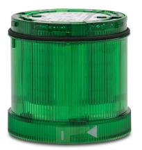
WERMA LED light element, 70mm diameter, green, rotating (120rpm) light function, 24 VAC/VDC, colored lens, IP65.
