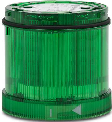
WERMA LED light element, 70mm diameter, green, rotating (120rpm) light function, 24 VAC/VDC, colored lens, IP65.
