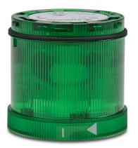
WERMA LED light element, 70mm diameter, green, flashing (1 Hz ON for 2x10ms) light function, 24 VDC, colored lens, IP65.
