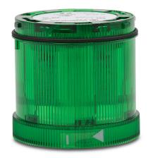
WERMA LED light element, 70mm diameter, green, blinking (1 Hz ON for 550ms) light function, 24 VAC/VDC, colored lens, IP65.
