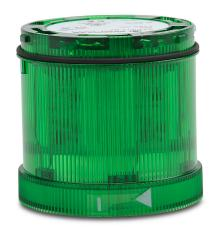
WERMA LED light element, 70mm diameter, green, blinking (1 Hz ON for 550ms) light function, 115 VAC, colored lens, IP65.
