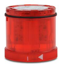
WERMA LED light element, 70mm diameter, red, blinking (1 Hz ON for 550ms) light function, 115 VAC, colored lens, IP65.
