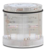
WERMA Xenon tube light element, 70mm diameter, clear/white, flashing strobe (1 Hz ON for 10ms) light function, 115 VAC, clear lens, IP65.
