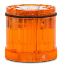
WERMA Xenon tube light element, 70mm diameter, yellow, flashing strobe (1 Hz ON for 10ms) light function, 115 VAC, colored lens, IP65.
