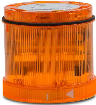
WERMA Xenon tube light element, 70mm diameter, yellow, flashing strobe (1 Hz ON for 10ms) light function, 24 VDC, colored lens, IP65.
