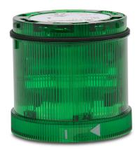
WERMA Xenon tube light element, 70mm diameter, green, flashing strobe (1 Hz ON for 10ms) light function, 24 VDC, colored lens, IP65.
