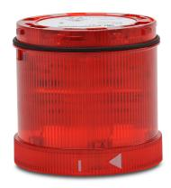
WERMA Xenon tube light element, 70mm diameter, red, flashing strobe (1 Hz ON for 10ms) light function, 115 VAC, colored lens, IP65.
