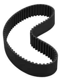
SureMotion timing belt, 8mm 8M pitch, 30mm wide, 80 tooth, 640mm pitch length (circumference), neoprene, fiberglass reinforced.
