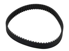
SureMotion timing belt, 8mm 8M pitch, 20mm wide, 80 tooth, 640mm pitch length (circumference), neoprene, fiberglass reinforced.
