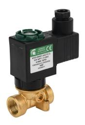
Spartan solenoid valve, 2-way, 2-position, N.C., low lead brass body, 3/8in female NPT inlet(s), 3/8in female NPT outlet(s), Cv=0.72, 50 psi maximum operating pressure, 120 VAC operating voltage, 18mm DIN style wiring plug.
