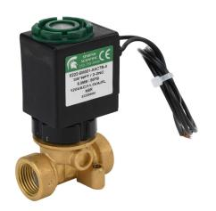
Spartan solenoid valve, 2-way, 2-position, N.C., low lead brass body, 3/8in female NPT inlet(s), 3/8in female NPT outlet(s), Cv=0.72, 50 psi maximum operating pressure, 120 VAC operating voltage, 18in 22 AWG pigtail.
