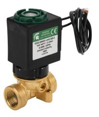
Spartan solenoid valve, 2-way, 2-position, N.C., low lead brass body, 3/8in female NPT inlet(s), 3/8in female NPT outlet(s), Cv=0.72, 40 psi maximum operating pressure, 24 VDC operating voltage, 18in 22 AWG pigtail.
