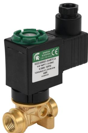
Spartan solenoid valve, 2-way, 2-position, N.C., low lead brass body, 1/4in female NPT inlet(s), 1/4in female NPT outlet(s), Cv=0.72, 50 psi maximum operating pressure, 120 VAC operating voltage, 18mm DIN style wiring plug.
