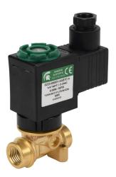
Spartan solenoid valve, 2-way, 2-position, N.C., low lead brass body, 1/4in female NPT inlet(s), 1/4in female NPT outlet(s), Cv=0.72, 50 psi maximum operating pressure, 120 VAC operating voltage, 18mm DIN style wiring plug.
