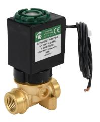
Spartan solenoid valve, 2-way, 2-position, N.C., low lead brass body, 1/4in female NPT inlet(s), 1/4in female NPT outlet(s), Cv=0.72, 50 psi maximum operating pressure, 120 VAC operating voltage, 18in 22 AWG pigtail.
