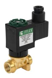
Spartan solenoid valve, 2-way, 2-position, N.C., low lead brass body, 1/4in female NPT inlet(s), 1/4in female NPT outlet(s), Cv=0.72, 40 psi maximum operating pressure, 24 VDC operating voltage, 18mm DIN style wiring plug.
