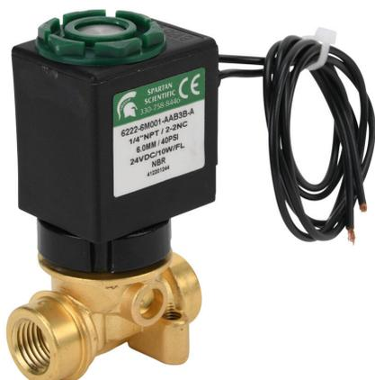
Spartan solenoid valve, 2-way, 2-position, N.C., low lead brass body, 1/4in female NPT inlet(s), 1/4in female NPT outlet(s), Cv=0.72, 40 psi maximum operating pressure, 24 VDC operating voltage, 18in 22 AWG pigtail.
