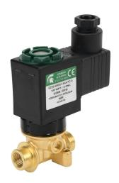
Spartan solenoid valve, 2-way, 2-position, N.C., low lead brass body, 1/8in female NPT inlet(s), 1/8in female NPT outlet(s), Cv=0.72, 50 psi maximum operating pressure, 120 VAC operating voltage, 18mm DIN style wiring plug.
