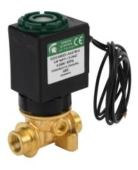
Spartan solenoid valve, 2-way, 2-position, N.C., low lead brass body, 1/8in female NPT inlet(s), 1/8in female NPT outlet(s), Cv=0.72, 50 psi maximum operating pressure, 120 VAC operating voltage, 18in 22 AWG pigtail.
