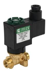
Spartan solenoid valve, 2-way, 2-position, N.C., low lead brass body, 1/8in female NPT inlet(s), 1/8in female NPT outlet(s), Cv=0.72, 40 psi maximum operating pressure, 24 VDC operating voltage, 18mm DIN style wiring plug.
