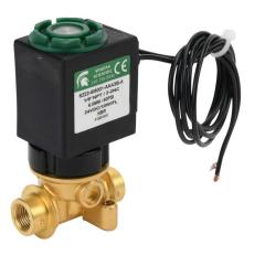
Spartan solenoid valve, 2-way, 2-position, N.C., low lead brass body, 1/8in female NPT inlet(s), 1/8in female NPT outlet(s), Cv=0.72, 40 psi maximum operating pressure, 24 VDC operating voltage, 18in 22 AWG pigtail.
