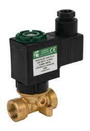
Spartan solenoid valve, 2-way, 2-position, N.C., low lead brass body, 3/8in female NPT inlet(s), 3/8in female NPT outlet(s), Cv=0.61, 80 psi maximum operating pressure, 120 VAC operating voltage, 18mm DIN style wiring plug.
