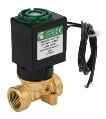
Spartan solenoid valve, 2-way, 2-position, N.C., low lead brass body, 3/8in female NPT inlet(s), 3/8in female NPT outlet(s), Cv=0.61, 80 psi maximum operating pressure, 120 VAC operating voltage, 18in 22 AWG pigtail.
