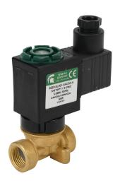
Spartan solenoid valve, 2-way, 2-position, N.C., low lead brass body, 3/8in female NPT inlet(s), 3/8in female NPT outlet(s), Cv=0.61, 60 psi maximum operating pressure, 24 VDC operating voltage, 18mm DIN style wiring plug.
