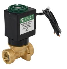
Spartan solenoid valve, 2-way, 2-position, N.C., low lead brass body, 3/8in female NPT inlet(s), 3/8in female NPT outlet(s), Cv=0.61, 60 psi maximum operating pressure, 24 VDC operating voltage, 18in 22 AWG pigtail.
