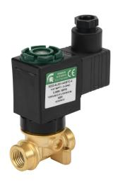
Spartan solenoid valve, 2-way, 2-position, N.C., low lead brass body, 1/4in female NPT inlet(s), 1/4in female NPT outlet(s), Cv=0.61, 80 psi maximum operating pressure, 120 VAC operating voltage, 18mm DIN style wiring plug.
