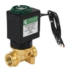
Spartan solenoid valve, 2-way, 2-position, N.C., low lead brass body, 1/4in female NPT inlet(s), 1/4in female NPT outlet(s), Cv=0.61, 80 psi maximum operating pressure, 120 VAC operating voltage, 18in 22 AWG pigtail.
