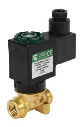
Spartan solenoid valve, 2-way, 2-position, N.C., low lead brass body, 1/4in female NPT inlet(s), 1/4in female NPT outlet(s), Cv=0.61, 60 psi maximum operating pressure, 24 VDC operating voltage, 18mm DIN style wiring plug.
