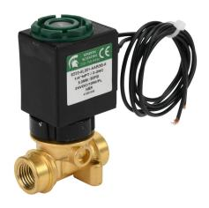
Spartan solenoid valve, 2-way, 2-position, N.C., low lead brass body, 1/4in female NPT inlet(s), 1/4in female NPT outlet(s), Cv=0.61, 60 psi maximum operating pressure, 24 VDC operating voltage, 18in 22 AWG pigtail.
