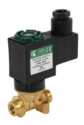
Spartan solenoid valve, 2-way, 2-position, N.C., low lead brass body, 1/8in female NPT inlet(s), 1/8in female NPT outlet(s), Cv=0.61, 80 psi maximum operating pressure, 120 VAC operating voltage, 18mm DIN style wiring plug.
